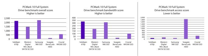
[Figure 4. PCMark 10 Full System Drive benchmark results]
