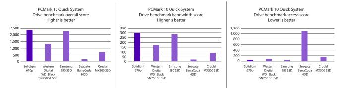
[Figure 3. PCMark 10 Quick System Drive benchmark results]
